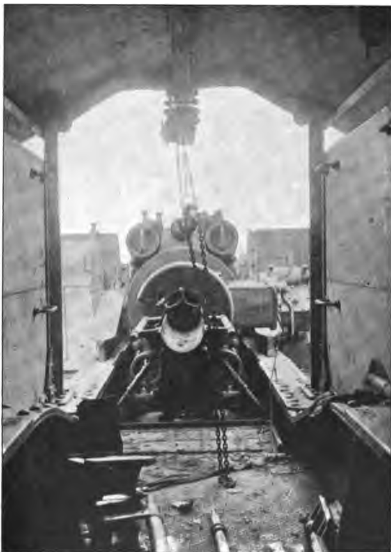
BREECH MECHANISM AND LOADING APPARATUS OF THE 210-MM. GERMAN MOUNT.
